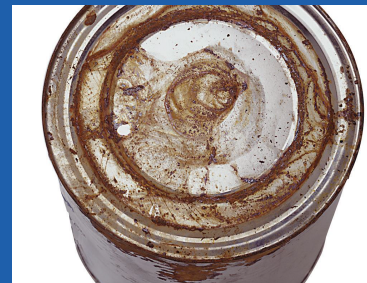
Excessive and pitted rust
