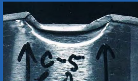
Severe double seam dent plate fracture
