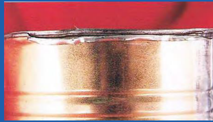
False seam with loss of hermetic seal
